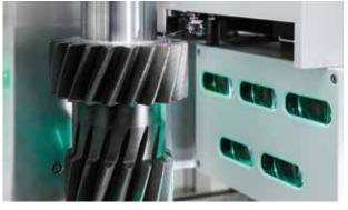
Probing system TSP for Opticline C and CA series
