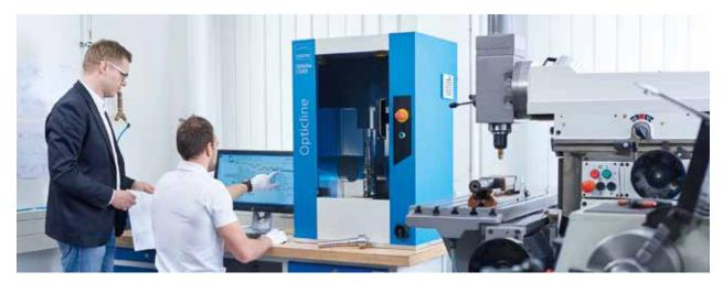
Opticline CS305 for cost-effective measurement of turned parts
