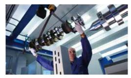
Use in production, loading a crank shaft with operator self-inspection
