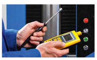
Workpiece temperature detection
