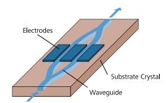
Schematic layout of an integrated-optical amplitude modulator
