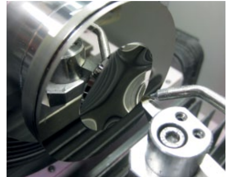
FIG. 3: Machined mold positioned at the ultra precision machine.
