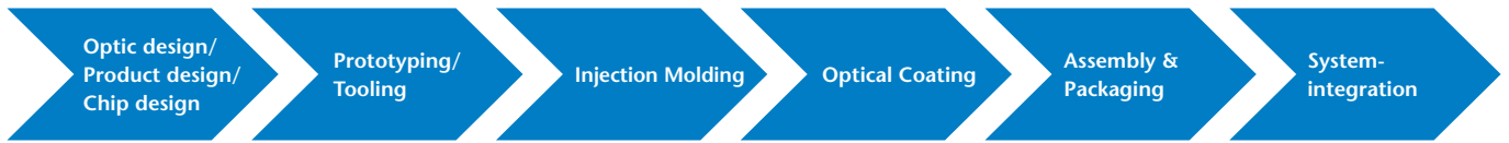
FIG. 1: Process chain for realizing optoelectronic systems in high volumes.
