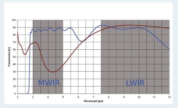
Fig2: Multispectral anti-reflective coating of single-layer DLC coating (red) and Hybrid-DLC coating (blue)
